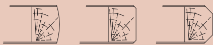
Hardwood leading edges Core material from MDF or Chipboard Laminated and balanced
